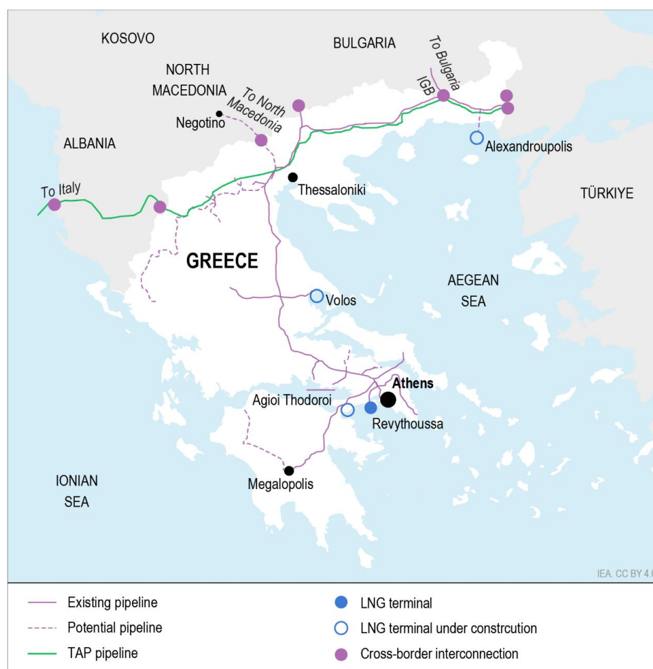
Figure 4-5: The natural gas grid in Greece
