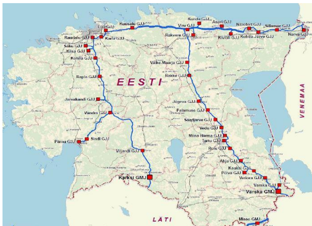
Figure 3-5. Natural gas grid infrastructure in Estonia
